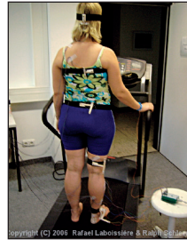
3D marker movement recording
